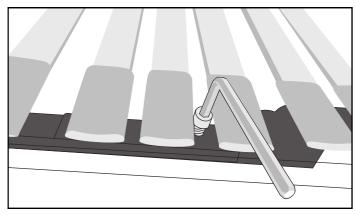
**NOTE**: Do NOT tighten bolts securely until all (4) bolts have been installed into connecting rods
