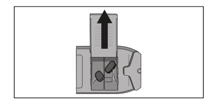
Insert the two 9V batteries (included) into the compartment and slide the cover back on.
