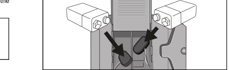
Insert one end of the DC cord into the power supply. Insert the other end with locking clip into the cable coming from the control box. Lock the connection using the locking clip.
