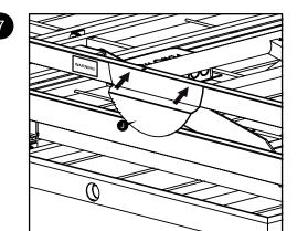
Plug in elevation motor cable into control box's
